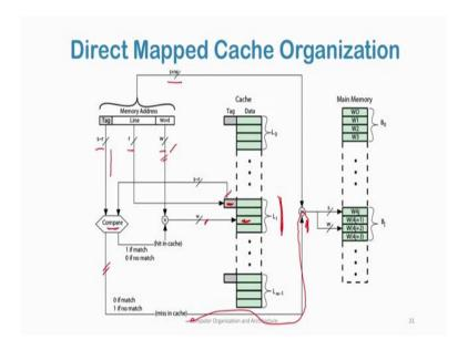
So, this figure shows the organization of a direct mapped cache. We see that the memory address consists of s + w bits. The tag is s - r bits long. The cache line index, the cache index the cache is indexed by an r bit length quantity and the each word within a particular block or line is identified by the by this word offset here by this word offset ok.
